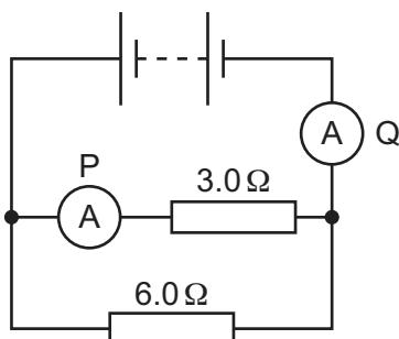
What is the combined resistance of the two resistors and which ammeter has the greater reading?
